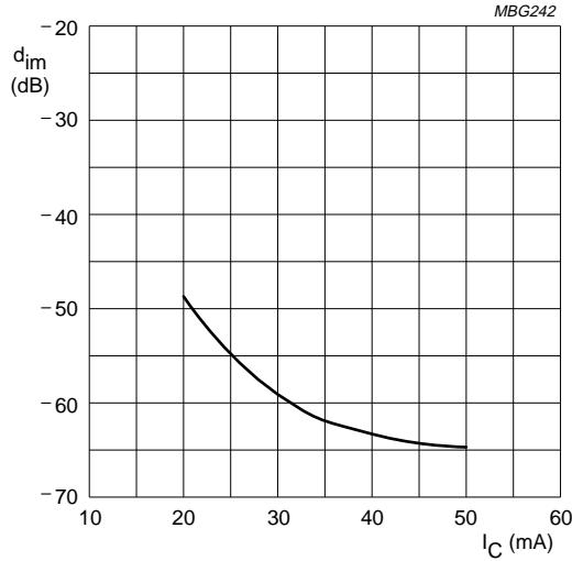
$V_{CE} = 8$  V;  $V_o = 475$  mV;  $R_L = 50 \Omega$ .
