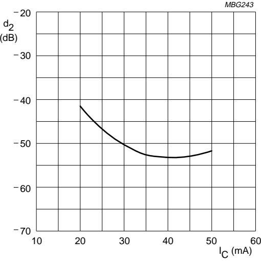
$V_{CE} = 8$  V;  $V_o = 225$  mV;  $R_L = 50 \Omega$ ;  $f_{(p+q)} = 810$  MHz;  $T_{amb} = 25$  °C.
